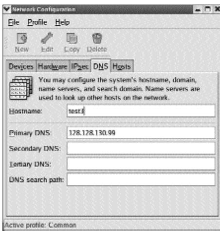
Use the Network Configuration tool to enter the IP address and other network information
